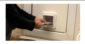
If you find that the read range of your SureFlap is compromised by the metal present in your door. (range test results of 12-22cm) you will need to follow metal mounting instructions to leave a gap between the metal and the tunnel of the SureFlap
